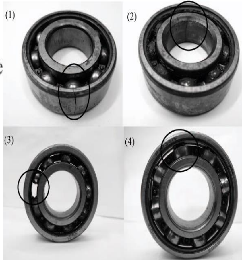
Fig. 3 (a): Photos of defective bearings used on shaft-side (6205), (1) Outerrace, (2) Innerrace, (3) Cage, and (4) Ball
